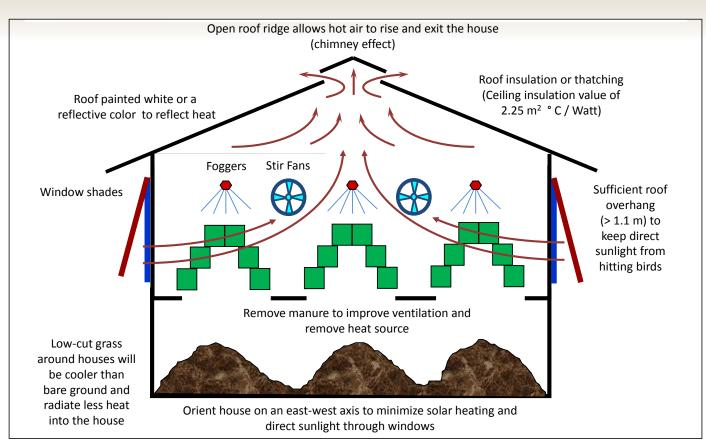
Figure 7. Open house design for reducing heat stress.
